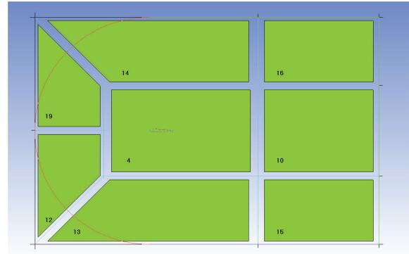
Abbildung 2: Blöcke in ICEM CFD [Luc22, S.10]
