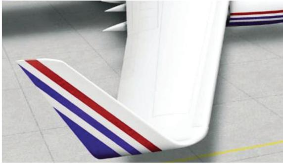
Figure 2: Blended winglet configuration [6]
