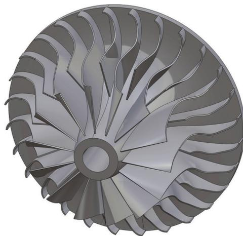
Figure 1: Impeller of the centrifugal compressor – designed with CATIA V5-6R2012
