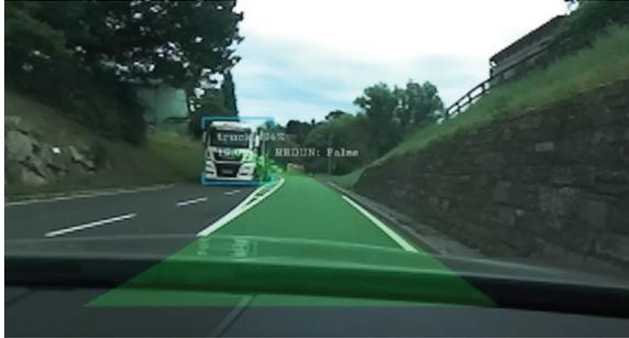
Figure 7: Lane detection: detected lanes are displayed in green
